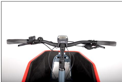
**Bild:** Handlebars with handlebar stem (including Speedlifter)
